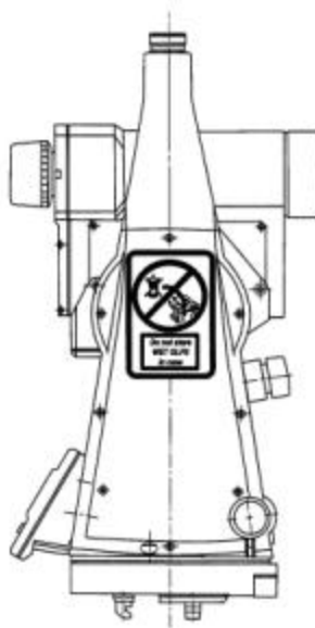
Figure 3-10. Theodolite Instruction Label
